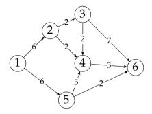
The nodes are routers, the edges are communications links; associated with each node is a capacity — node 1 can communicate to node 2 at as much as 6 Mbps, node 2 can communicate to node 4 at up to 2 Mbps, etc.
