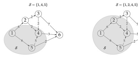
The edges in the cut are  $1 \rightarrow 2, 4 \rightarrow 6$ , and  $5 \rightarrow 6$  the capacity of this cut is 6 + 3 + 2 = 11.
